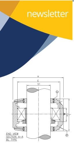
BMI manufactures pillow blocks in two main styles: SAF and SDAF. Other types are available on "make to order" basis. The larger SDAF block is suggested for extreme heavy duty applications.
