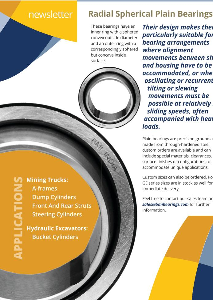
Their design makes them particularly suitable for bearing arrangements where alignment movements between shaft and housing have to be accommodated, or where oscillating or recurrent tilting or slewing movements must be possible at relatively slow sliding speeds, often accompanied with heavy loads.
